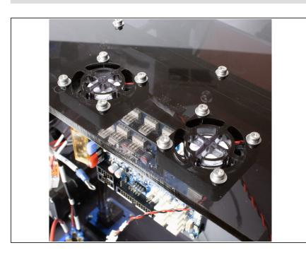
Using (4) M3 x 20 socket head screws, M3 washers, and M3 nuts, install the (2) panel fans under the rear panel.
