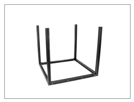
Use (1) M3 x 8mm socket head screws to attach each of the (4) 270mm upright extrusions to the corner cubes on the bottom frame assembly.
