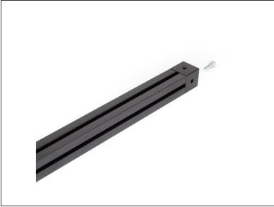
• Use (1) M3 x 8mm socket head screw to the 270mm bottom left extrusion. Note the orientation of the corner cube.
