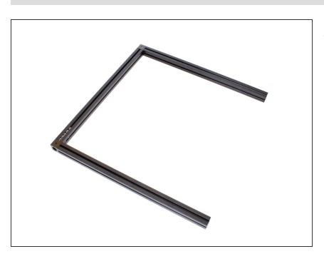
Attach bottom (2) 270mm front and bottom back extrusions using (1) M3 x 8mm socket head screw each.
