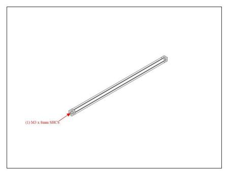
Attach Second Corner Cube to Top Right Extrusion using (1) M3 x 8mm socket cap head screw.
