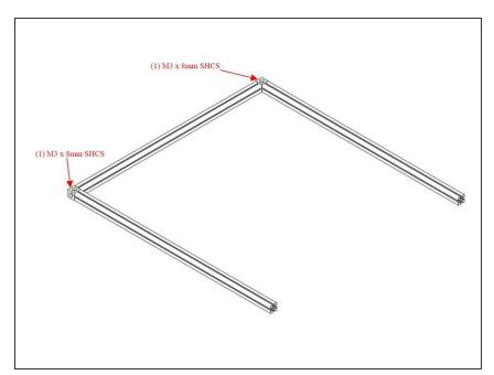
Attach the (2) 460mm Top Front and Top Back Extrusions using (1) M3 x 8mm socket cap head screw each.
