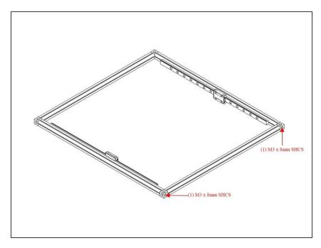
Attach Top Right Extrusion to the rest of the Top Extrusion Assembly using (2) M3 x 8mm socket cap head screws.
