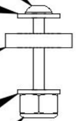
**Step 1 — Assemble the Bolt Stacks for Attaching the bed**
