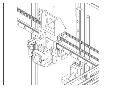
Insert a length of PTFE into the hotend, at least 91mm long. (You want around 45mm sticking out of the hotend when it's fully seated)
