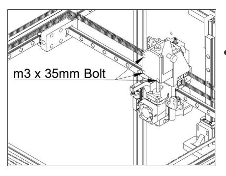
Fasten the BMG and stepper together on the extruder mount using (3) M3 x 35mm bolts. (These bolts come with the BMG)
