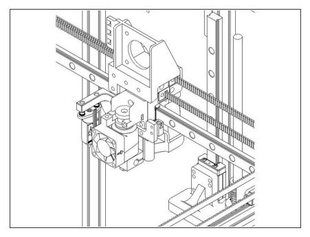
The E3D v6 should have been assembled already. It fits into the groovemount adapter as shown. It's best to turn it so the heat block is not too close to the fan shroud.
