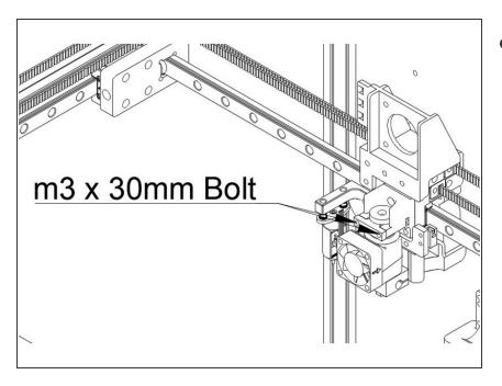
Use the hotend retainer (a small printed part) to fasten in the E3d v6 using (2) m3 x 30mm button head bolts.
